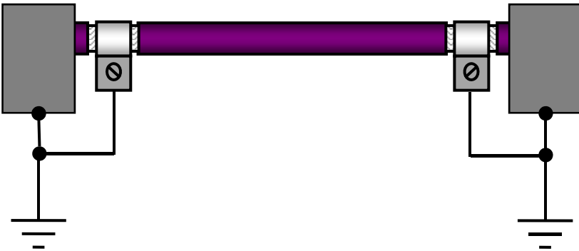
Figure 3-32 Standard grounding concept for PROFIBUS
